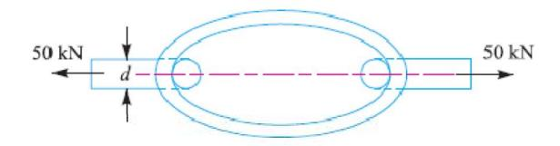
**Solution.** Given:  $P = 50 \text{ kN} = 50 \times 10^3 \text{ N}$ ;  $\sigma_t = 75 \text{ MPa} = 75 \text{ N/mm}^2$
