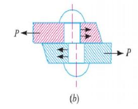
when the shearing takes place at **two cross-sections** of the rivet), then the rivets are said to be in **double shear**. In such a case, the area resisting the shear off the rivet,
