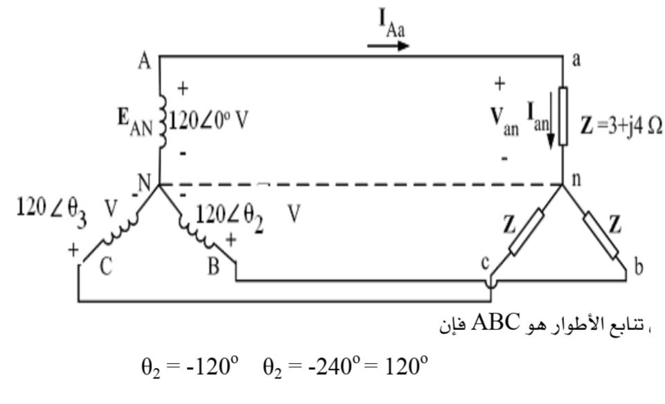
$V_{AB} = V_{BC} = V_{CA} = \sqrt{3} \times 120 = 208 \text{ V}$
