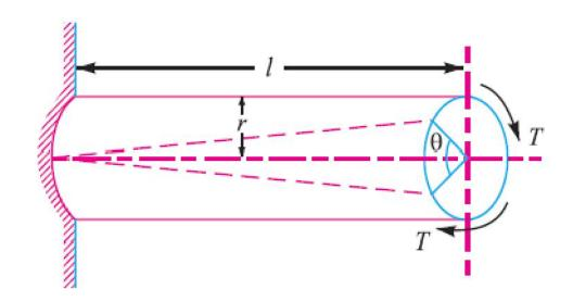
Consider a shaft fixed at one end and subjected to a torque (T) at the other end as shown in Figure. As a result of this torque, every cross-section of the shaft is subjected to torsional shear stress. The maximum torsional shear stress at the outer surface of the shaft may be obtained from the following equation:
